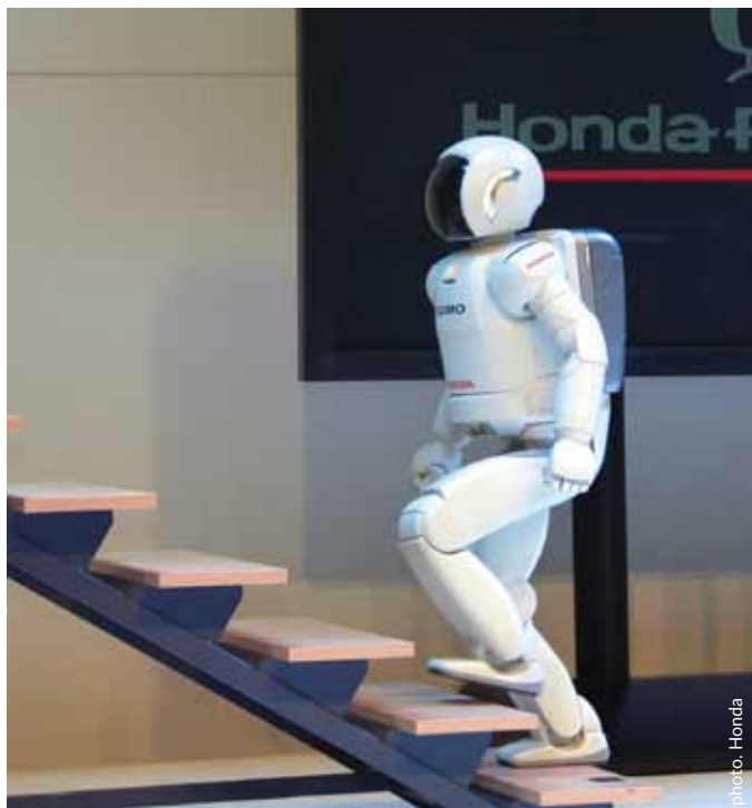
Honda's ASIMO robot is considered the most advanced humanoid in the world; ASIMO (Advanced Step In Innovative Mobility).
